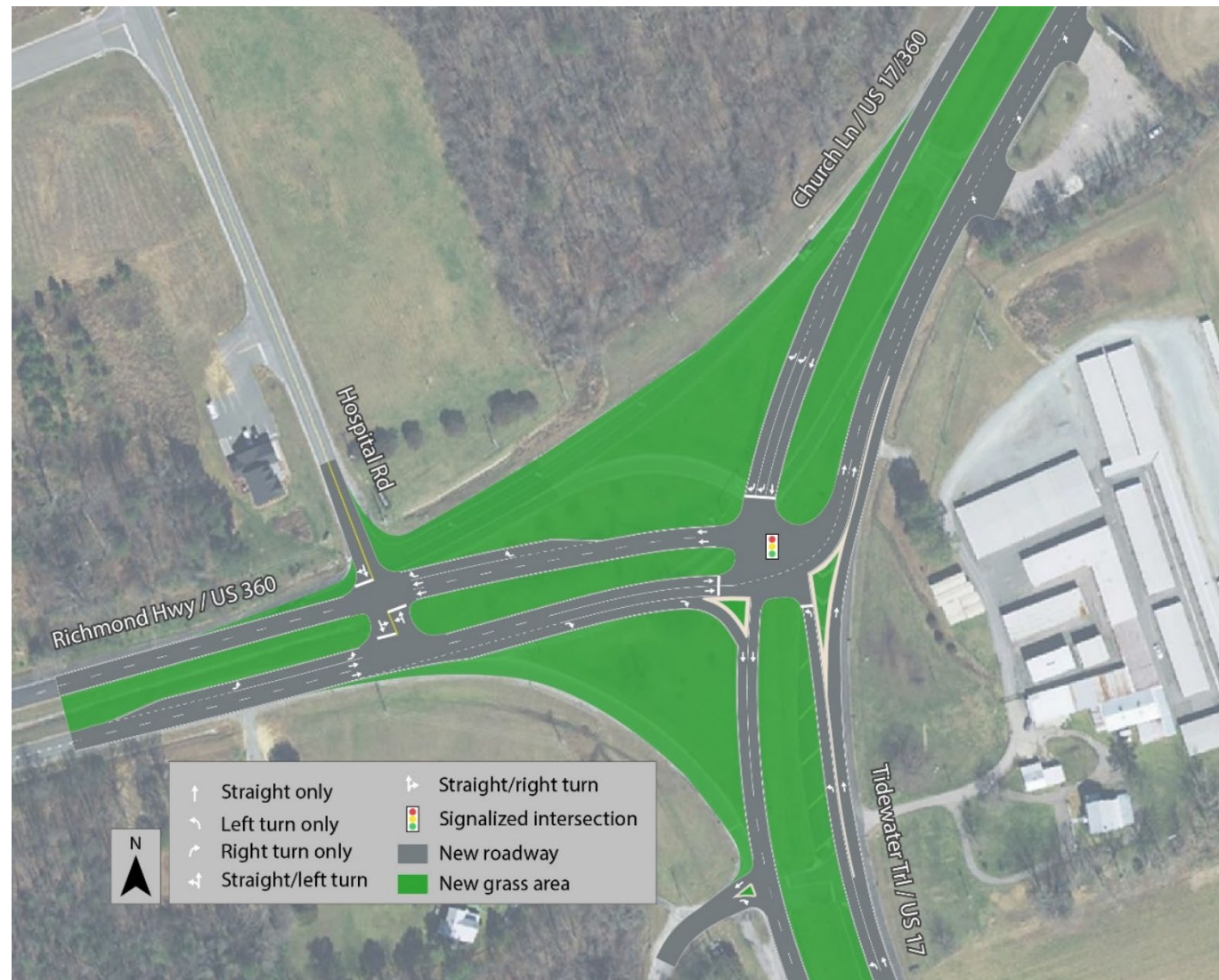
FIGURE 48: BRAYS FORK CONTINUOUS GREEN-T
