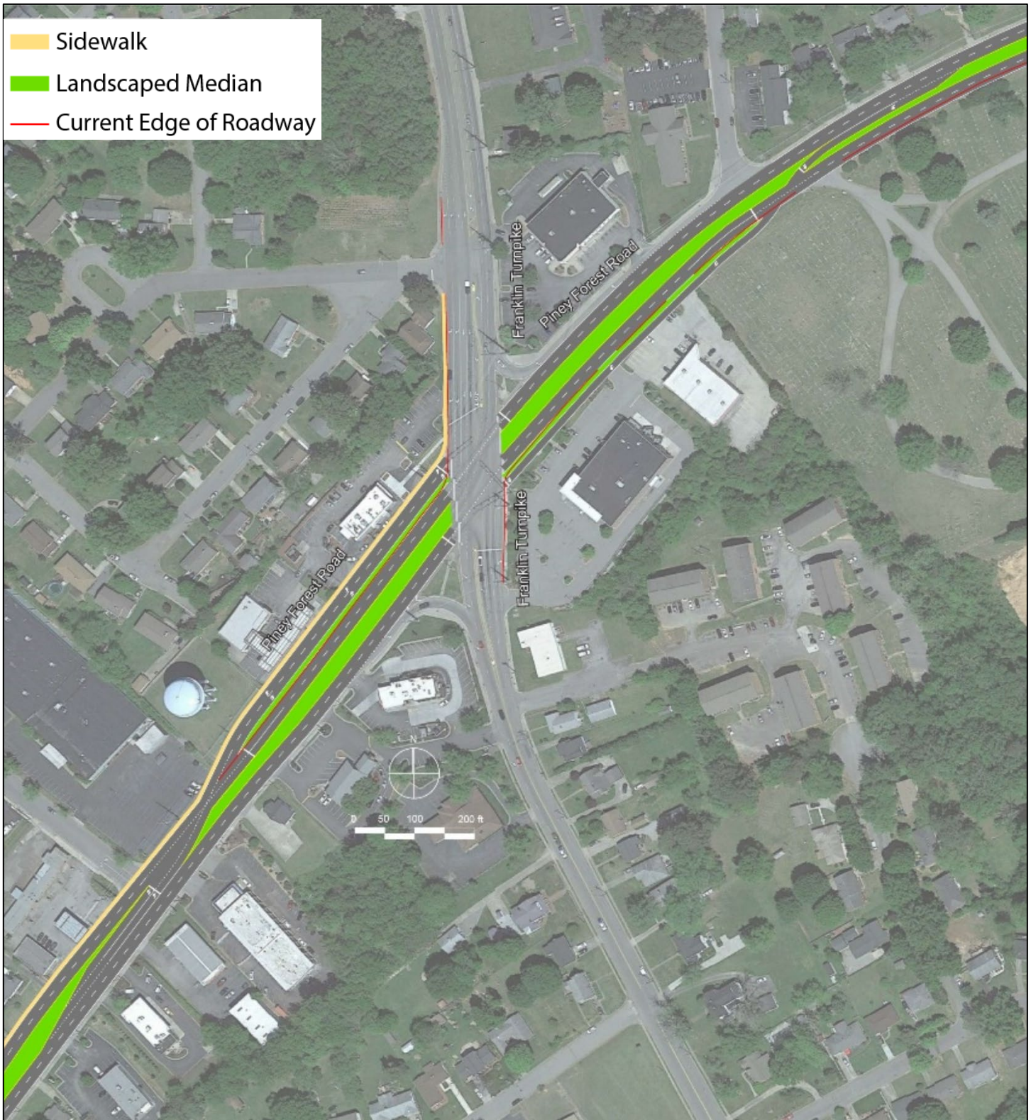
FIGURE 48: FRANKLIN TURNPIKE DISPLACED LEFT TURN INTERSECTION
