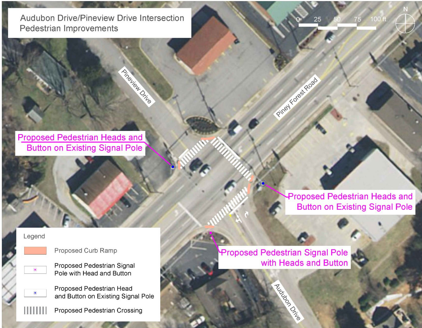
FIGURE 42: AUDUBON DRIVE INTERSECTION PEDESTRIAN IMPROVEMENTS
