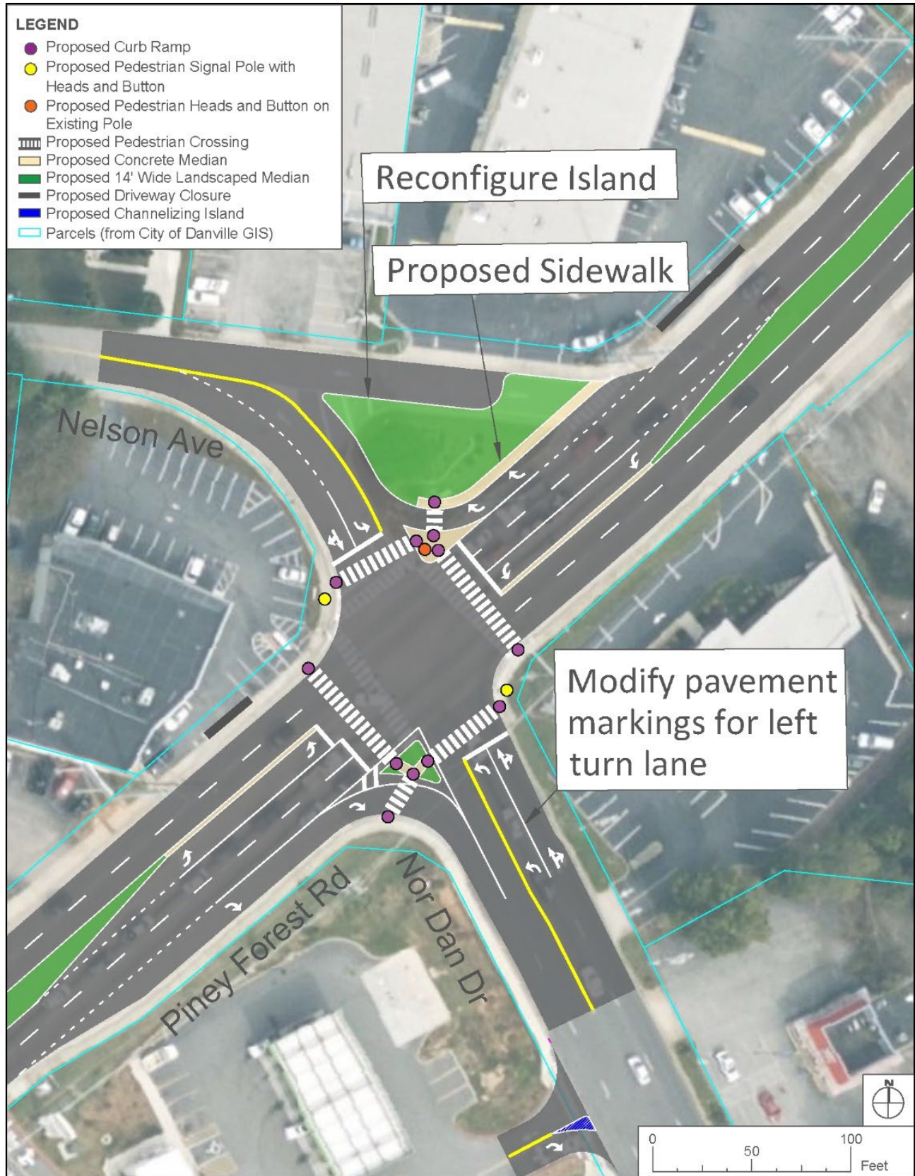
FIGURE 50: NELSON AVENUE/NOR DAN DRIVE INTERSECTION IMPROVEMENTS
